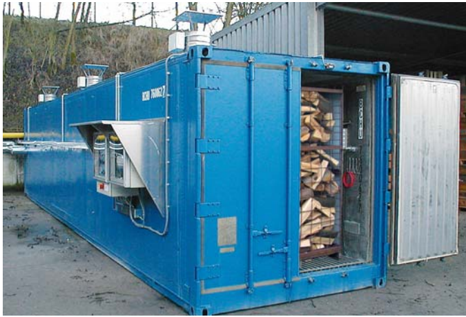
Skeleton boxes with 1 m 3 of firewood each in a small drying kiln (container solution).
