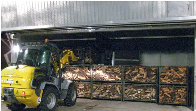
Loading of a drying kiln with skeleton boxes filled with firewood.
