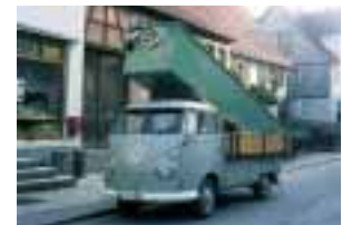
"Transportable" Lauber wood dryer in the past (1968).
